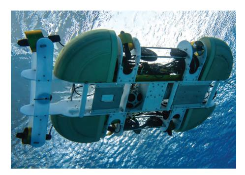
Xplorer is a subsea pipeline inspection-class autonomous underwater vehicle (AUV) developed by a Thai engineering team. Xplorer is able to measure the contact Cathodic Protection (CP), a unique and advanced solution compared to existing commonly available products in the market. Moreover, the Xplorer does not require Non-DP Vessel to support its operation, which enables it to offer significant savings in operational cost by reducing vessel size.
